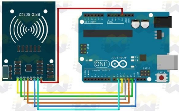
Fig. 4. Arduino-RFID Link Representation.
